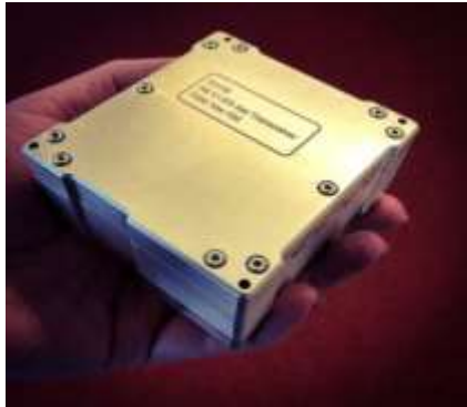
R6 VDES Satellite Transceiver for LEO
